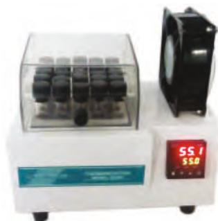
It is a closed reflux digester used for digestion applications & can also be used for COD estimation with very small quantity of sample.
